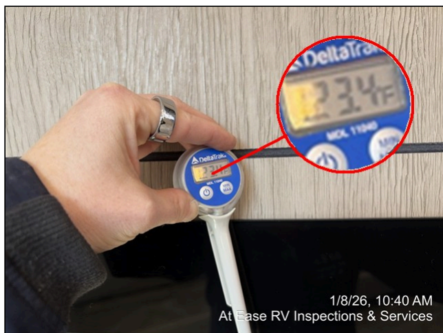
17.21 Item 1 (Picture) Fireplace output temp
