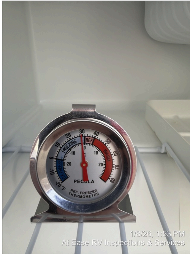
22.0 Item 1 (Picture) Outside fridge/freezer temp
