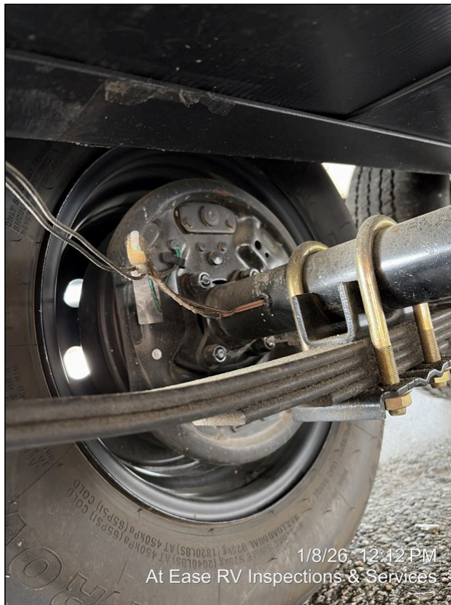
12.4 Item 1 (Picture) U Bolts, brake wires, etc
