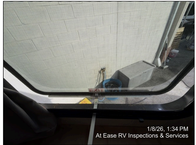
20.30 Item 2 (Picture) Top bunk emergency exit window
