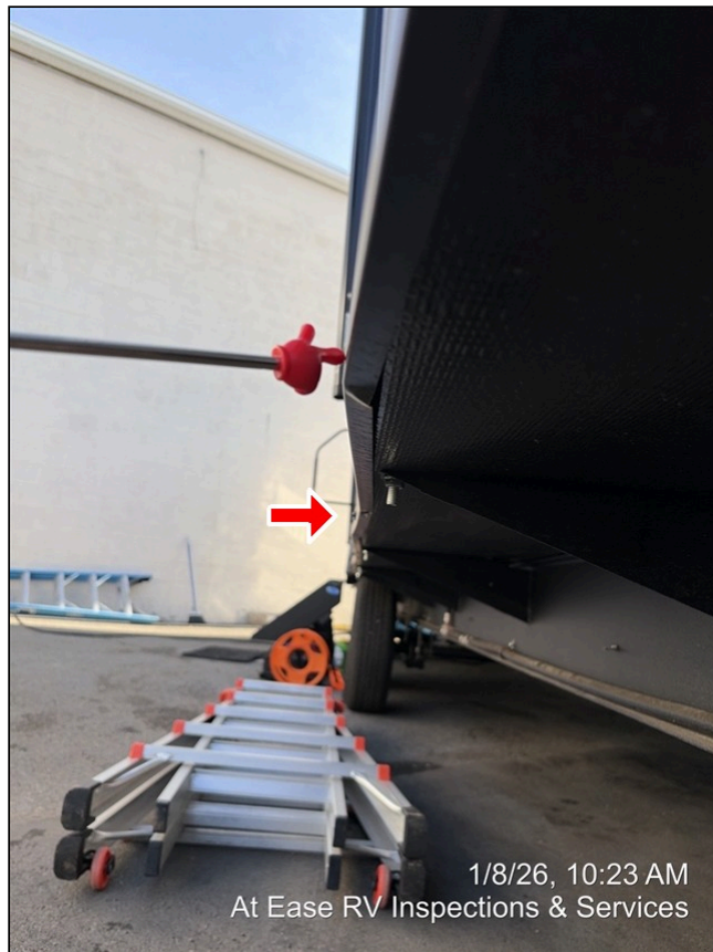
7.0.B Item 1 (Picture) Bends in metal skin
