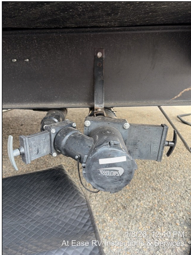
15.15 Item 1 (Picture) Primary dump valves
